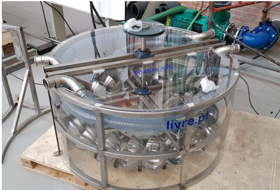
Figure 4.5: New Water wheel for SilkHouse application.
