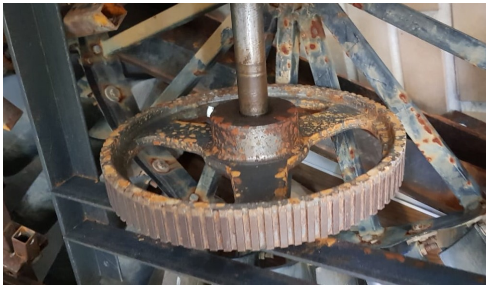
Figure 4.4: Water wheel and its oxidation.
