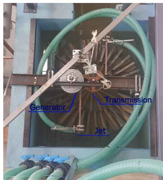
Figure 3.3: Top view of Water wheel.
