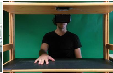
Figure 2. Oculus Rift and Leap Motion from [11].
