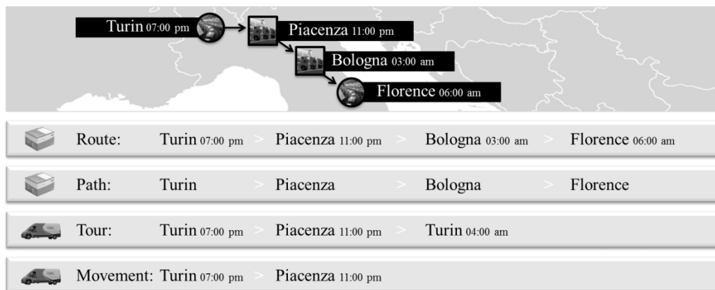
Figure 38: The path and route illustrate the movements of packages from their origin (e.g., Turin) to their final destination (e.g., Florence) and the vehicle movements. The path is the subset of a route that excludes drop-off times. A movement connects two successive locations and is a subset of a tour.
