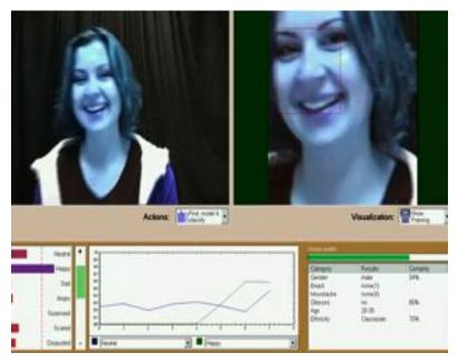
Figure 2: A screenshot of FaceReader during the AM session. The horizontal green bar (right) shows that the picture quality (input to the FaceReader) is excellent. The vertical green bar (left) shows the perceived valence and the pink horizontal bars (extreme left) show the emotion categories. In this case, FaceReader categorizes the face as 'happy' with a high degree of certainty (purple bar crossing the dotted vertical line).
