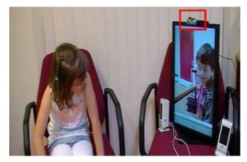
Figure 4: Mutual gaze Condition: Webcam on the top of the side screen where partner's live video is shown (a rectangle shows the camera position)
