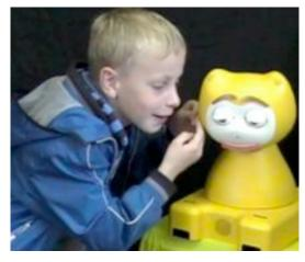
Figure 5: iCat showing frown expression (with head down, lower eyelids, curved lips) and the child showing sympathy to iCat after losing a game
