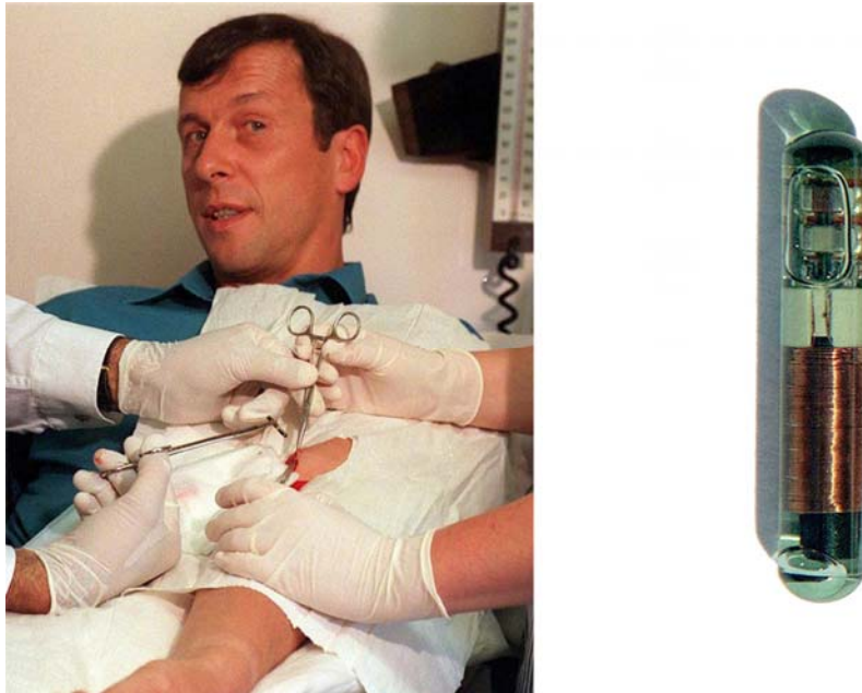
Figure 2: A 2cm long RFID tag (shown right) is invasively implanted into a healthy volunteer during a research program conducted in 1998.
