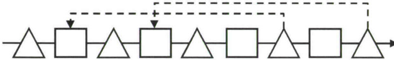
Figure 11. A pull structure that does not match the typology of known systems
