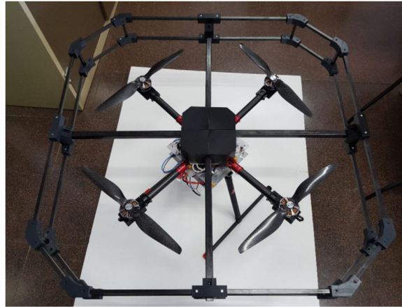
Figure 3. Prototype UAV platform developed as a base for a sample collector UAV part of the UAV sensing network.
