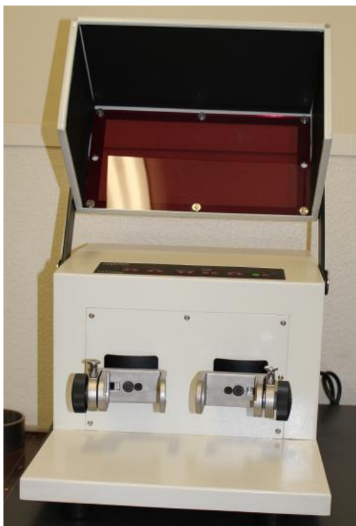
Figure 3.1. A photograph of the shaker mill used for mechanical studies.
