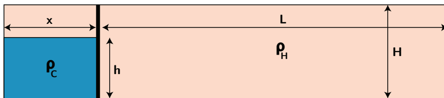
FIGURE 1.3: Schematic of a general lock-exchange experiment. Blue color corresponds to heavy (cold) fluid while the pink color represents light (hot) fluid. Lock gate is represented as a vertical dark line.
