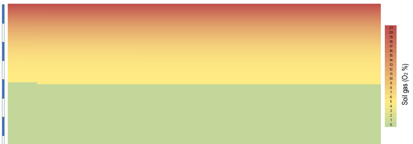
Figure 7-4: 2D Finite Difference Soil Gas Diffusion Model –Fixed Diffusion Coefficient, 3m GWT, no cracks.
