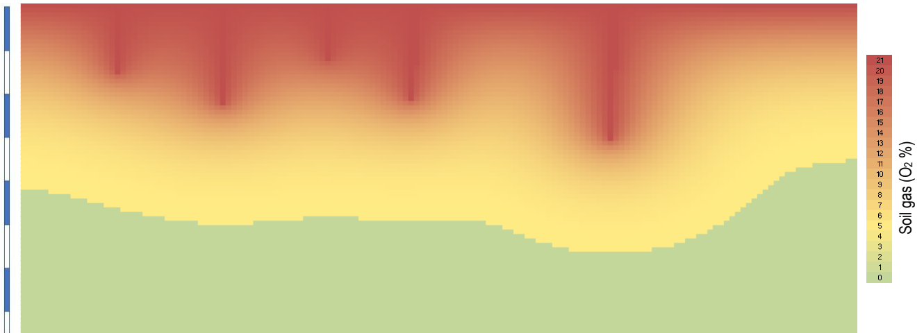
Figure 7-6: 2D Finite Difference Soil Gas Diffusion Model –Fixed Diffusion Coefficient, TSF crack model, 3m GWT.
