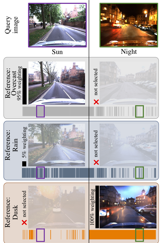
Fig. 1. Given a query image, Bayesian Selective Fusion selects and fuses informative reference images to find the best place match. Left: Given sunny query images, our approach selects images from the overcast and rain reference sets (frequently discarding the dusk images), and fuses them according to their likelihood (higher transparency indicates lower likelihood; see also black bars). Right: Given night query images, our approach selects images from the dusk reference set (frequently discarding the overcast and rain images) since they are perceptually most similar to night images. Note however that when dusk images offer limited visual information (e.g., due to sun glare), additional images from the rain and overcast references are selected and fused.
