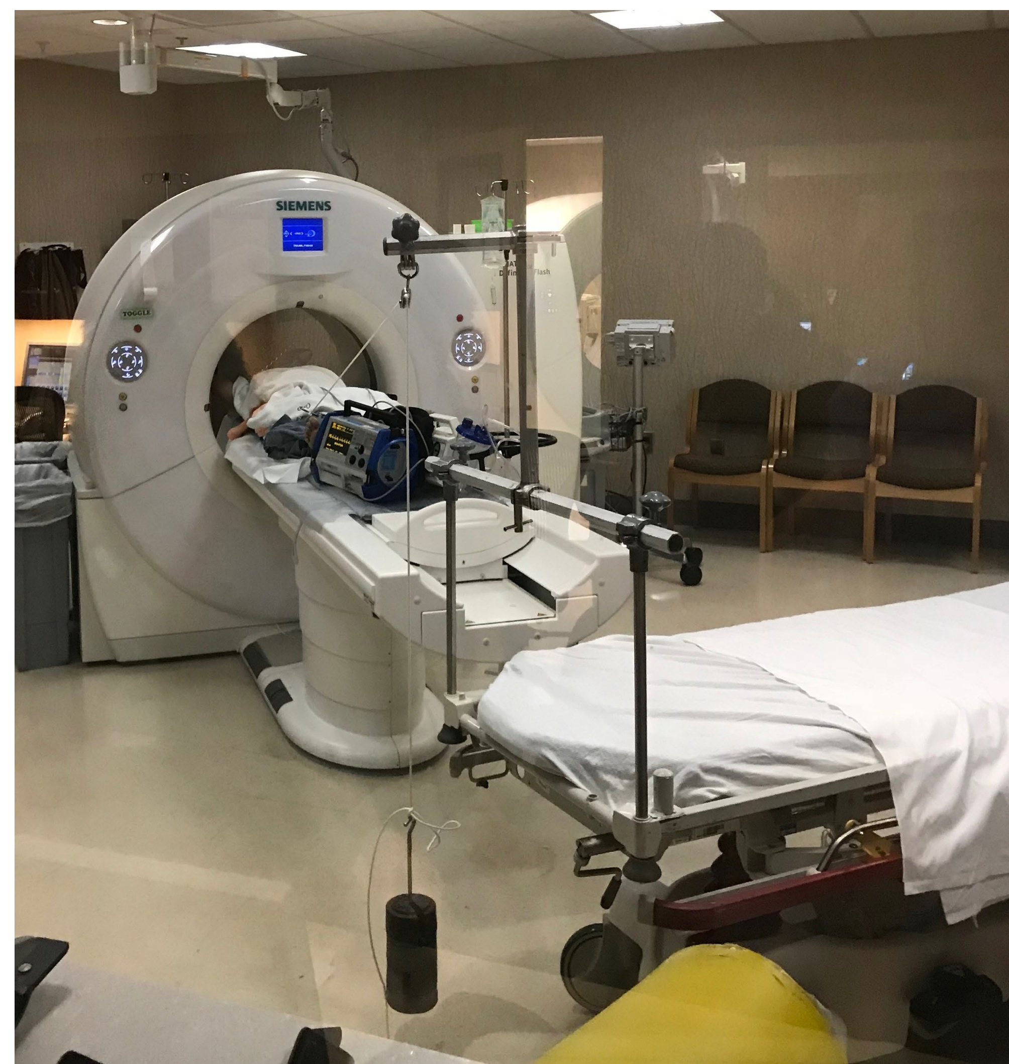
Figure 1: Technique #1 utilizing patient bed as counter-weight
