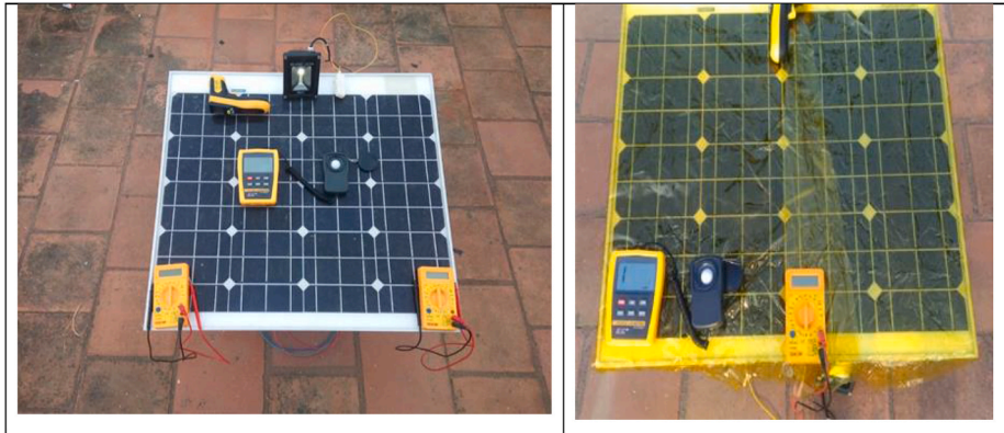
Fig. 3. Experimental arrangements of the photovoltaic module without and with a colour filter. (For interpretation of the references to colour in this figure legend, the reader is referred to the Web version of this article.)
