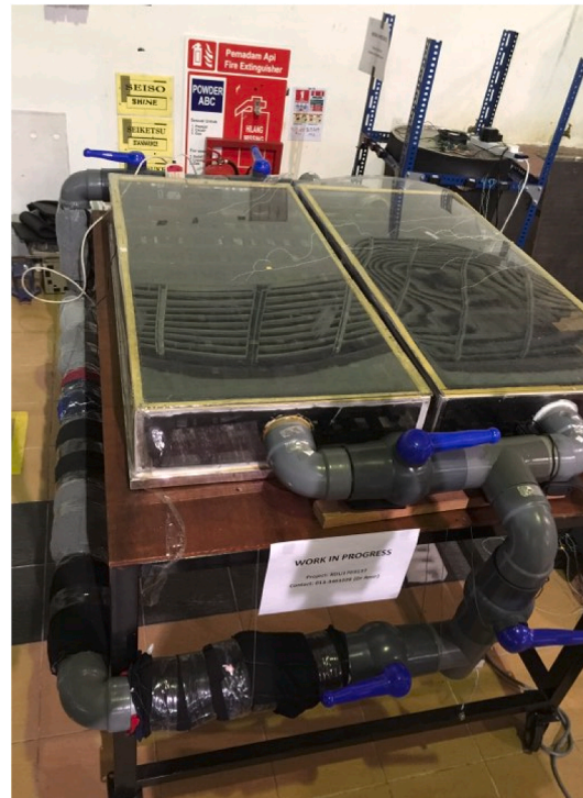
Fig. 2. Solar collectors in series and parallel configurations.
