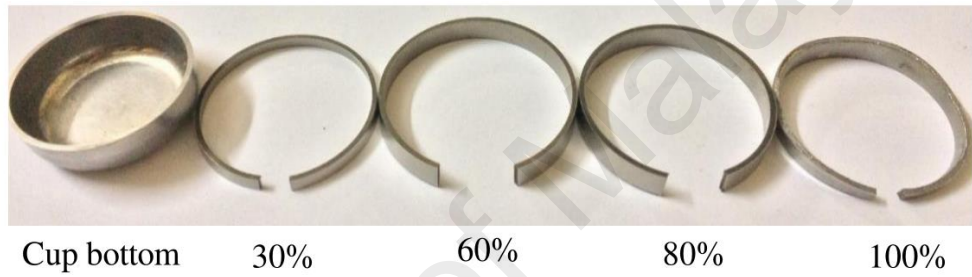
Figure 3.8: After: Slit cylindrical drawn cup into 5 different heights
