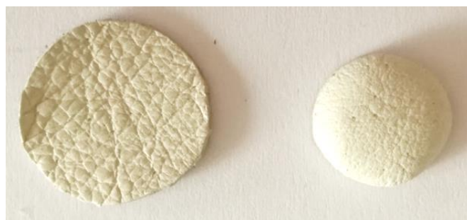
Fig. 12 Leather circle before and after heating [3]
