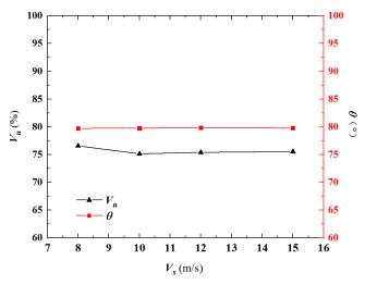
Fig. 14 Axial velocity distribution coefficient and weighted velocity average swirl angle under different ship speed conditions
