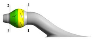
Fig. 8 Pressure measuring section
