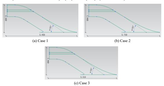
Fig. 17 Sketches of different cases involving inlet ducts with different lengths L
