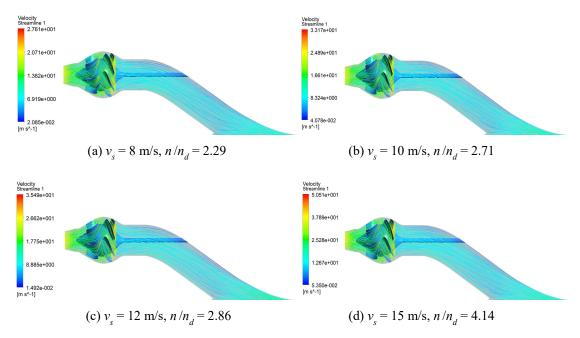
Fig. 15 Streamlines in the waterjet propulsion pump system under different ship speed conditions
