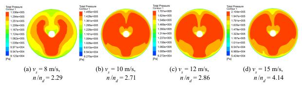
Fig. 13 Distribution of total pressure contour of the propulsion pump inlet under different ship speed conditions
