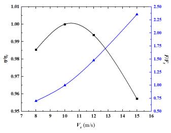
Fig. 16 System efficiency and thrust under different ship speed conditions
