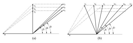
Fig. 12 Parallelogram rule of velocity at impeller inlet
