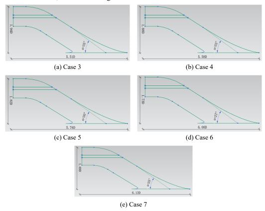
Fig. 19 Sketches of different cases involving inlet ducts with different dip angles  $\alpha$
