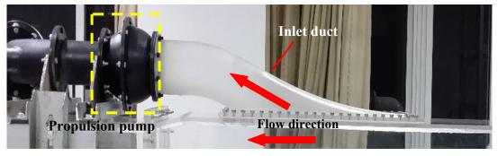
Fig. 7 Waterjet propulsion pumping system
