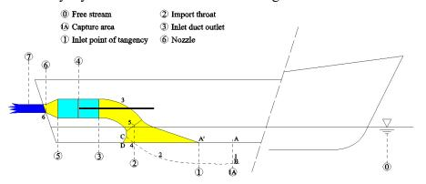
Fig. 10 24th ITTC definitions of standard locations of the waterjet propulsion system
