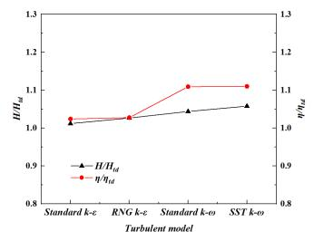
Fig. 5 Numerical and experimental results with different turbulence models
