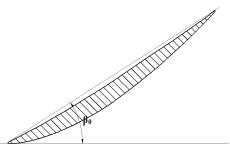
Fig. 11 Sketch of the setting angle of impeller blades
