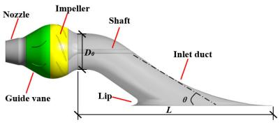
Fig. 2 Waterjet propulsion pump system
