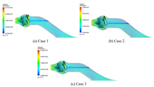
Fig. 18 Streamlines of different cases in the waterjet propulsion pump system
