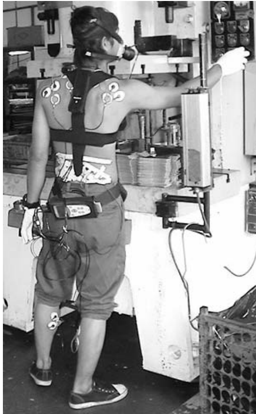
Figure 1: A Worker is Completely Attached with SEMG Electrodes
