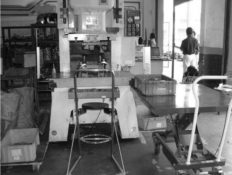
Figure 6: Improved Workstation Design – Intervention of Adjustable Table and Sit-stand Stool
