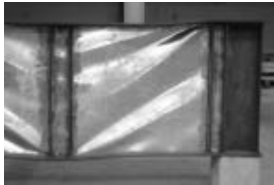
c) Buckling Mode of Specimen F550-1
