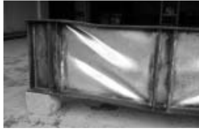
b) Buckling Mode of Specimen F450-1
