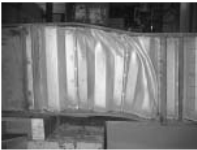
a) Zonal Buckling Mode of Specimens D350-1
