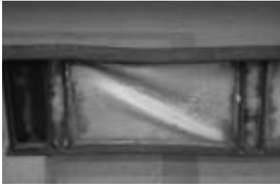
a) Buckling Mode of Specimen F350-1
