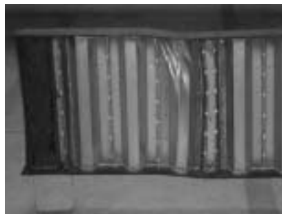
c) Zonal Buckling Mode of Specimens D550-1
