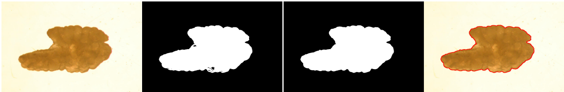
Figure 2.3: L-R: Original image; Initial segmentation using thresholding; segmentation after corrections; boundary overlaid on original image (boundary exaggerated for clarity)
