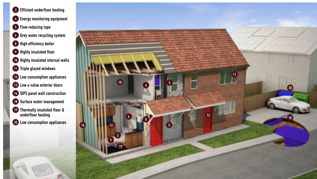
Figure 3.3b – Cross-section showing low-energy materials and renewable technologies installed at Trinity Close, Rackheath
