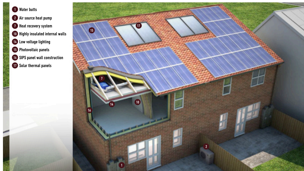
Figure 3.3a – Cross-section showing low-energy materials and renewable technologies installed at Trinity Close, Rackheath
