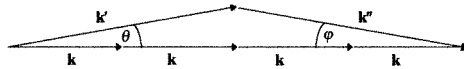
Figure 2. The arrows indicate the wavevectors for pump, k , probe, k' , and signal, k'' , for SWM.
