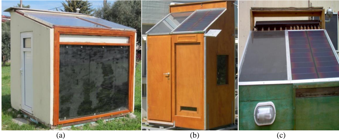
FIGURE 1. (a) The first IEB test cell with inbuilt south façade and solar roof. The pyranometer, provides signals for solar radiation prediction, (b) the second IEB pilot unit with a PV/T roof combined with the solar collector part, (c) another version of the same IEB unit where tubes with eco-Freon are attached in the PV back surface and in the solar collector construction.
