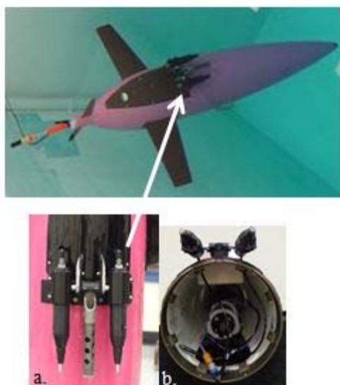
Fig. 1. Seaglider with microstructure sensing package. Inset a. is an enlargement of the MicroPod assembly. Inset b. shows the placement of the microstructure DataLogger pressure case inside the aft fairing of the glider in relation to the MicroPods.
