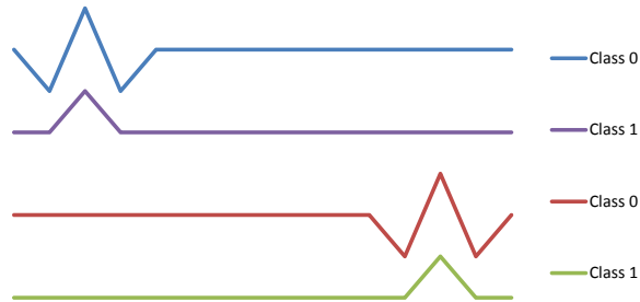
Figure 2.4: Time series of two different classes. A global approach will pair the series incorrectly, due to the offset in the time dimension. A local approach will pair the instances correctly, as the subsequences are exact matches.
