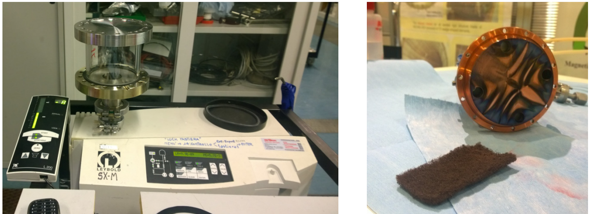
Figure 3.2 Leak test on Pyrex cylinder (left) and metal deposit on the cover of the rear multi-pole (right).
