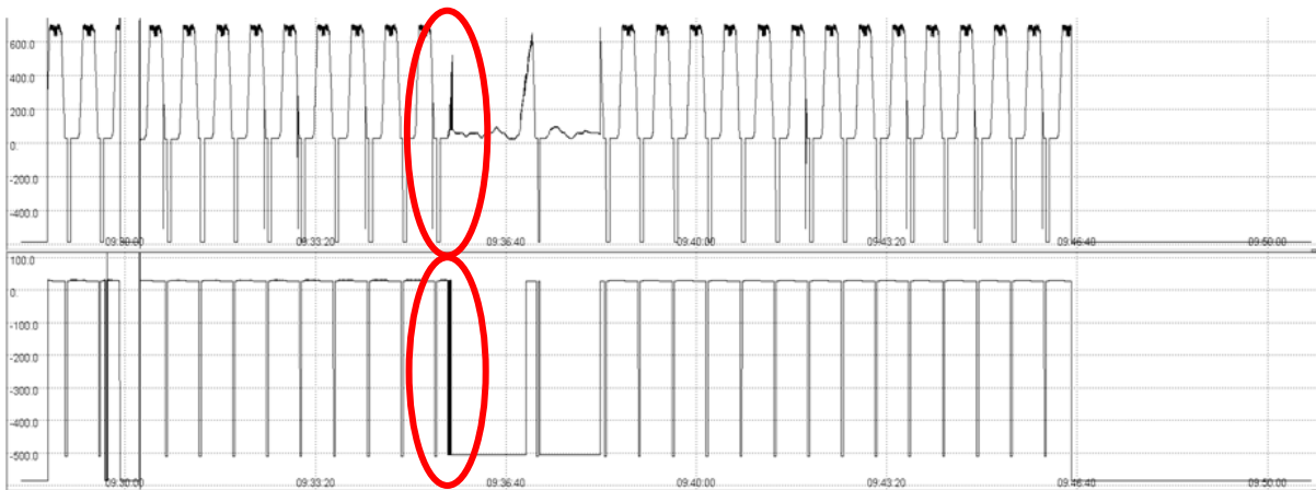
Figure 4.6 Fault detection signals from MAX31855.
