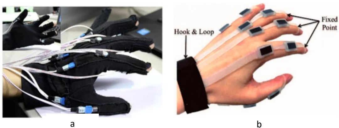
Figure 2.6: Data glove examples for a Sensor-based gesture recognition system. (a) Data glove presentation of Zheng [34] (b) Soft rubber data glove. [35]
