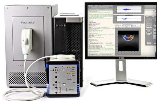
FIGURE 4.7: Verasonics Research System (adapted from [8]).
