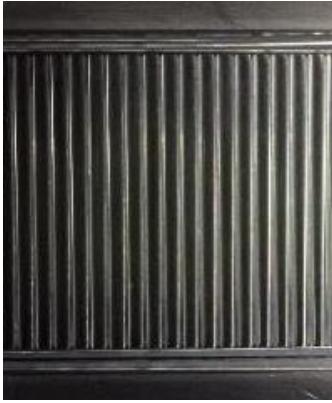
Fig. 2. Stainless steel plate incorporating the rectangular microchannels.
