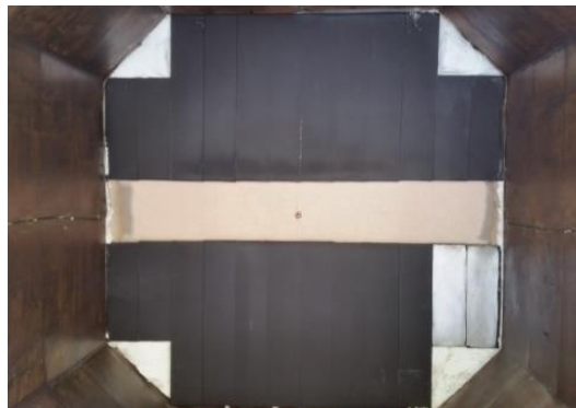
12 Figure 11 – Assemble of the rigid insulation panel with the flux sensor in the middle.
