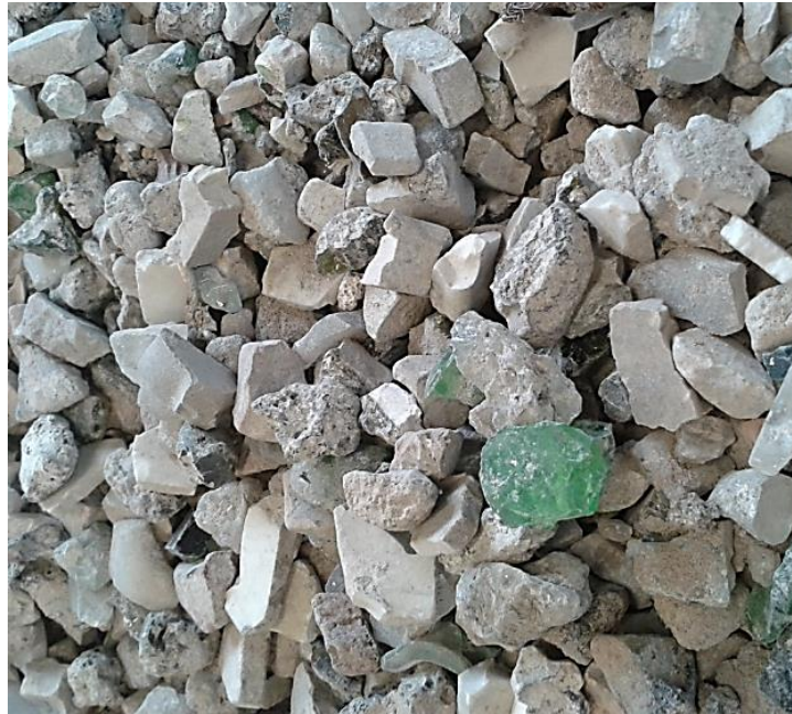
Figure 9.1: Appearance of the crushed sample after 100 revolutions and 10 steel balls;
