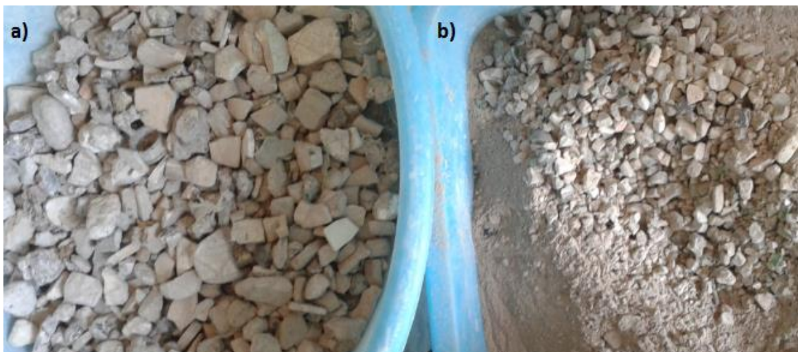
Figure 9.11: Comparison between the natural sample a) and that obtained after 500 revolutions b).
