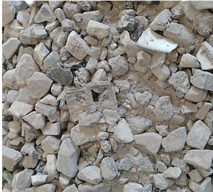
Figure 9.5: Appearance of the crushed sample after 500 revolutions and 10 steel balls;
