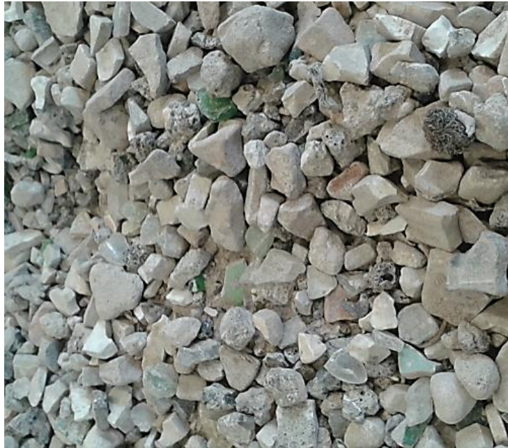
Figure 9.3: Appearance of the crushed sample after 200 revolutions and 10 steel balls;
