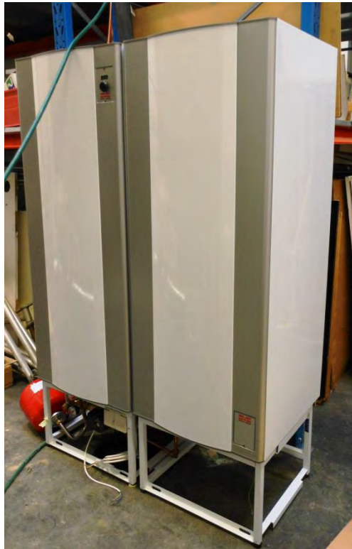
Figure 5.21 – Cold (on the left) and hot (on the right) water storage tanks
