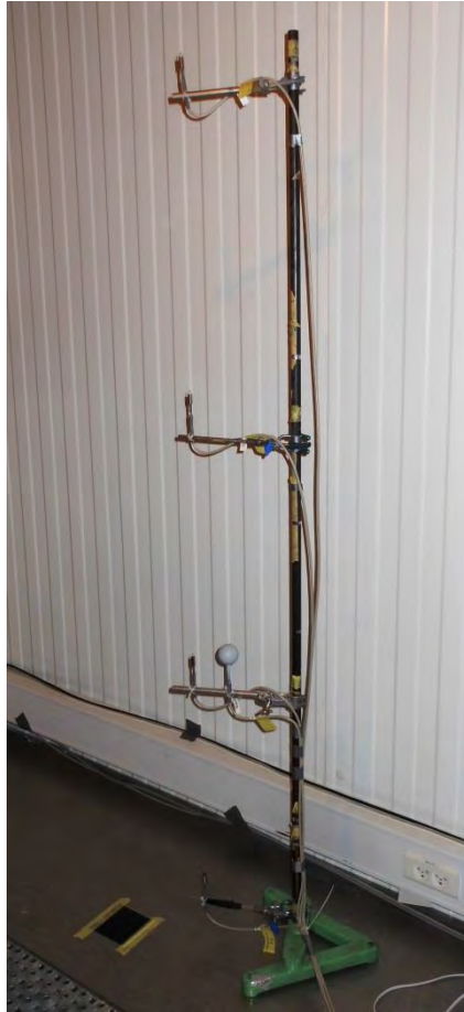
Figure 5.27 – Stand for measuring the air and the operative temperature inside the chamber
