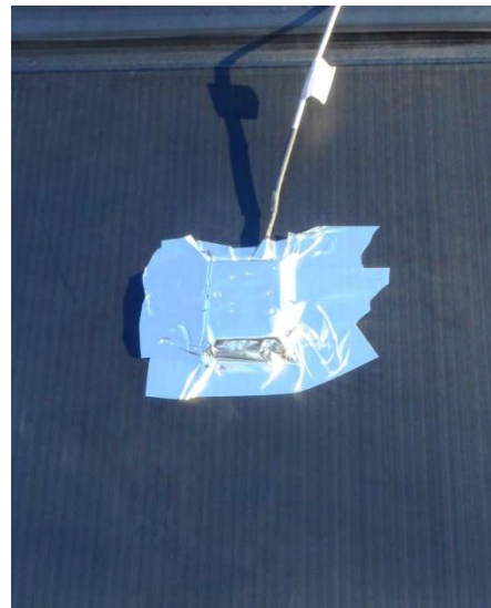
Figure 5.26 – Temperature sensor on the top surface of the unglazed collector
