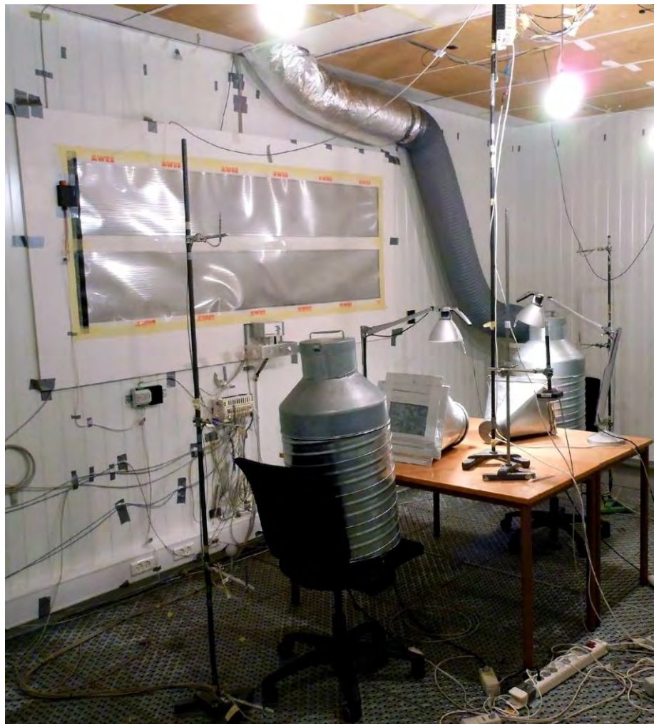
Figure 5.3 – Experimental setup of the climatic chamber
