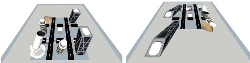
Figure 1. Two perspectives on the same presentation of a 3D model on a table; from one side the image looks correct, but from the other the image is distorted.
