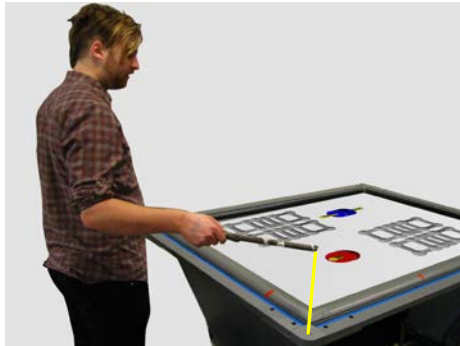
Figure 15. The participant specified perceived angle by manipulating the angle of a string attached to the right corner of the table and the tip of a wand (string highlighted in yellow). In this simulation, the participant is judging the red and yellow object shown at the quadrant of the surface closest to him.
