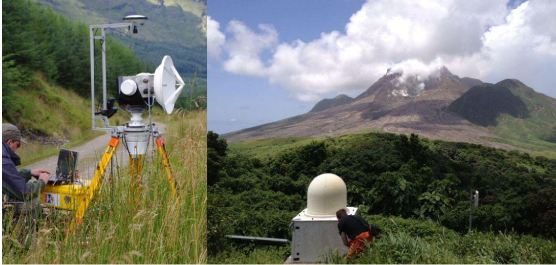
Fig. 1. AVTIS2 roving survey radar undergoing testing in Scotland, 2012 (left) and AVTIS3 under a radome at its remote telemetered installation at the Soufrière Hills Volcano (SHV), Montserrat, 2013 (right, photo Greg Scott). Both instruments are battery powered, gimbal mounted, rastered real-beam 94GHz FMCW radars designed to measure lava dome topography at a range of several km.
