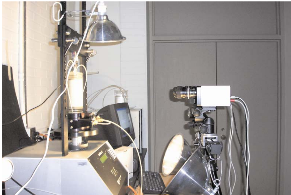
Figure 4.7 Triaxial test with 3D imaging system.
