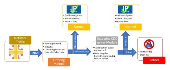
FIGURE 4. Block diagram for the proposed multilayer framework for botnet detection using machine learning algorithms.
