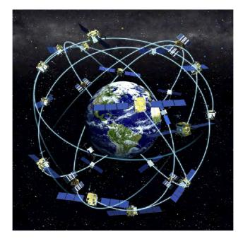
Figure 3.5: Baseline GPS constellation consisting of 24 satellites in orbital planes inclined at about 55° with respect to the Earths equatorial plane. Credit: National Oceanic and Atmospheric Administration (NOAA) (https://www.space.com/19794-navstar.html).
