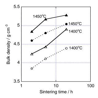
Fig. 5 Densification behaviors of LSO samples with 5 wt% BaF<sub>2</sub> addition (solid lines) and non-additive (broken lines) sintered at 1400° and 1450°C.
