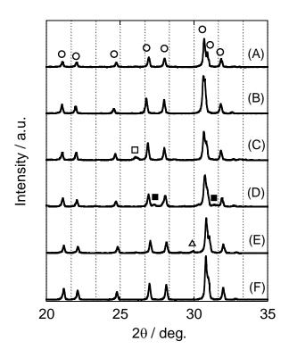
Fig. 2 XRD patterns of LSO samples sintered at 1450°C for 2 h (A) without additive and with 5 wt% of (B) BaF<sub>2</sub>, (C) AlF<sub>3</sub>, (D) NdF<sub>3</sub>, (E) CaF<sub>2</sub> and (F) NaF, showing ( $\circ$ ) LSO, ( $\square$ ) La<sub>2</sub>Si<sub>2</sub>O<sub>7</sub>, ( $\blacksquare$ ) La<sub>2</sub>SO<sub>5</sub> and ( $\Delta$ ) La<sub>2</sub>O<sub>3</sub>.
