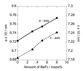
Fig. 6 Lattice parameter changes with an increasing amount of  $BaF_2$  addition for LSO samples sintered at 1450°C for 20 h.
