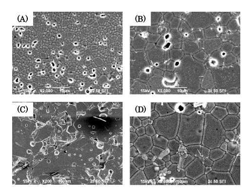
Fig. 3 Microstructures of LSO samples sintered at  $1450^{\circ}$ C for 20 h with (A) non-additive and the addition of 5 wt% (B) BaF<sub>2</sub>, (C) AlF<sub>3</sub> and (D) CaF<sub>2</sub>.
