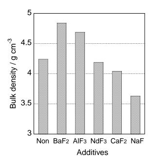
Fig. 1 Effect of various fluoride additives (5 wt%) on bulk densities of LSO samples sintered at 1450°C for 2 h.
