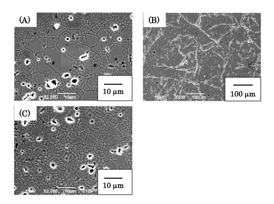
Fig. 4 Microstructure evolution of LSO samples with 5 wt% BAF sintered at (A) 1400°C for 20 h, (B) 1450°C for 2 h and (C) 1400°C for 5 h plus 1450°C for 5 h.
