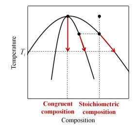
combinations are Al-Y and Y-Ca. The combination of Al-Ca can be excluded since both charges and crystallographic sites are different. Single crystals were accordingly grown using feed rods in which the chemical compositions are Y-rich for Ca (Y/Ca = 1.005/0.9925) and Al-rich for Y (Al/Y = 1.005/0.995). Polarizing microphotographs of the end portions are shown in Fig. 6. While the number of voids in the crystal grown
