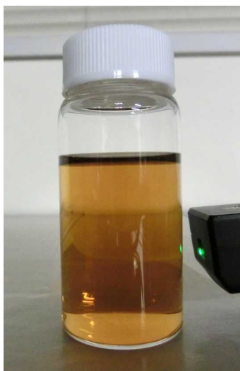
Fig. S2 Liquid phase of the reaction mixture after the hydrolysis of mix-milled cellulose containing Amberlyst. The solution was irradiated with a laser, but the Tyndall effect was hardly observed.
