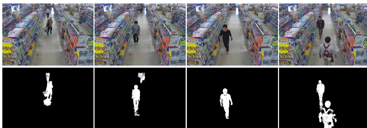
Fig. 10. Integrating CP3 method to an off-line supermarket shopper analysis system as its first step for person detection. In this supermarket scene, there is a large-area glass window facing the camera’s direction, so that the scene not only has light on/off, but also have sunlight change.
