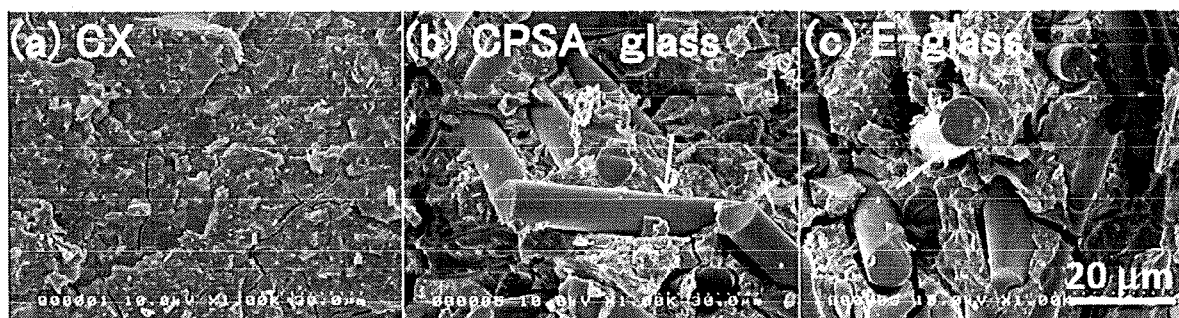
Figure 3 SEM photographs of fractured microstructures inside the set cements after DTS tests. (a) Set CX, (b) set cement containing 40 mass% short CPSA glass fibers and (c) set cement containing 40 mass % short E-glass fibers. Arrows shows short glass fibers.
