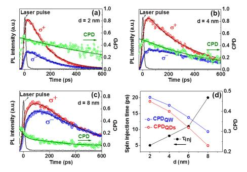
FIG. 3.  $\sigma^+$ - (red circles) and  $\sigma^-$ - (blue circles) polarized TRPL, and the CPD (green circles), fitted by the rate-equation calculations (solid lines) in the QDs with (a) d=2 nm, (b) d=4 nm, and (c) d=8 nm, respectively. (d) The barrier-thickness, d, dependences of the spin-injection time (filled black circles) and PL-CPDs (open circles).
