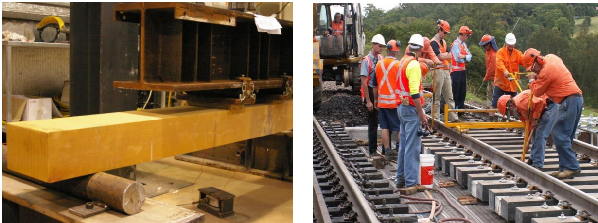
Figure 3: Glue-laminated fibre composite sandwich railway sleepers.
