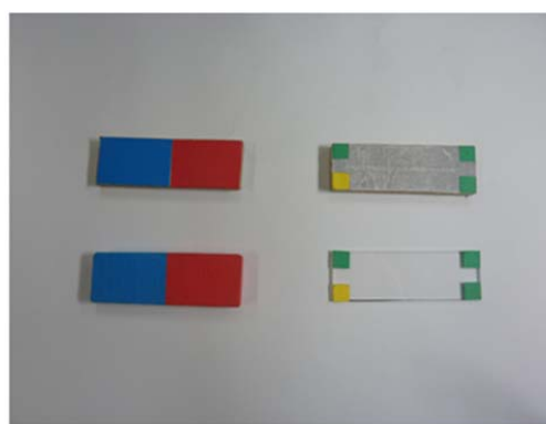
Fig. 5. Mocks representing bar magnets (left) and iron pieces (right). Left: blue and red color mean N- and S-pole, respectively. Right: yellow and green color mean markers. The yellow square markers represent the origin of the mocks, and it is recognized first. The green square markers represent the corners of the mocks. Using transparent material, a phenomenon on the display is observable even under the iron-piece mock.
