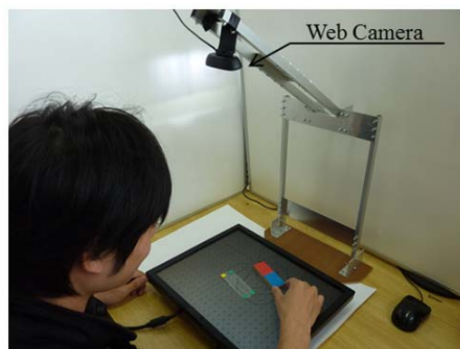
Fig. 4. Appearance of the proposed real-time visualization system. The proposed consists of a background monitor, a web camera, and some mocks. In the photo, one magnet and one iron mock are on the background monitor.
