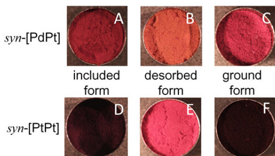
Fig. 4 Photographs of powder samples: A and D) vapour-included forms; B and E) desorbed forms; and C and F) ground forms, for syn -[PdPt] and syn -[PtPt], respectively.
