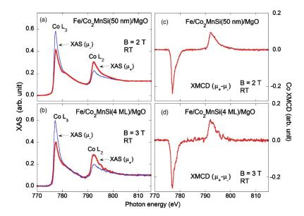
FIG. 1. (Color online) XAS (left panel) and XMCD (right panel) spectra at the  $\text{Co-}L_{2,3}$  edges for Fe/CMS (x nm) film/MgO, where x=50 nm for (a) and (c), and x=1.1 nm (=4 ML) for (b) and (d).
