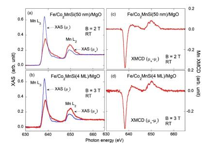
FIG. 2. (Color online) XAS (left panel) and XMCD (right panel) spectra at the Mn- $L_{2,3}$  edges for Fe/CMS (x nm) film/MgO, where x=50 nm for (a) and (c), and x=1.1 nm (=4 ML) for (b) and (d).
