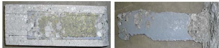
d. failure at primer to adhesive interface (B-2 series)
