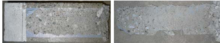
b. failure within concrete substrate (B-3 series)
