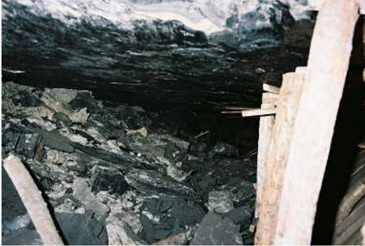
Fig. 11 Old roadway observed in Jobu Chuo No. 0 SD tailgate. Fallen rock slabs piled up on the heaved floor.
