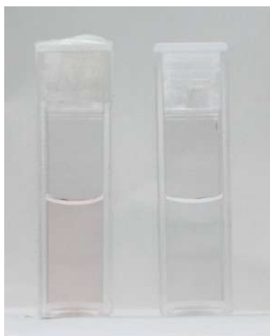
Fig. S3. Demonstration (run 1 in Fig 14) of the formation of gold particles using polymer 3 (entry 8). The left vial contains polymer 3 ( 46 \text{ unit}\cdot\text{mmol}\cdot\text{L}^{-1} , 1.8 \text{ mL} ) and \text{HAuCl}_4 aqueous solution ( 0.01 \text{ mol}\cdot\text{L}^{-1} ,
